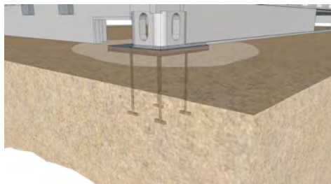
Concrete Footing Welded Container Base Plate
