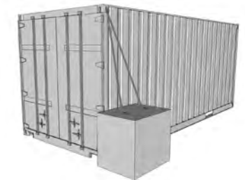
External Ballast Pre-Cast Concrete Block
